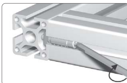
join the profiles and tighten the T-slot nut
