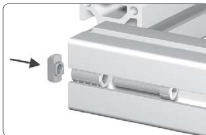
pre-mounting of the T-slot nut
