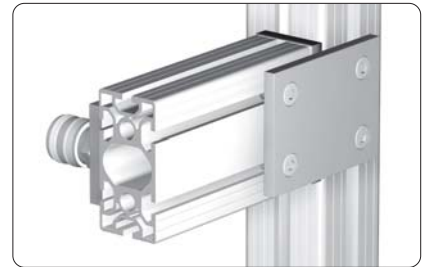
Connection of the pneumatic air manifold
