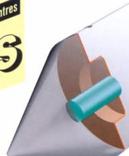
A safety core (German Federal Patent) is integrated in the carbide point of type SV, SVG. If the interface of carbide and base material becomes overstressed, e.g. through operating error or mishandling, the safety core prevents the carbide with the loaded component from slipping. Thus high consequential damage is avoided.
